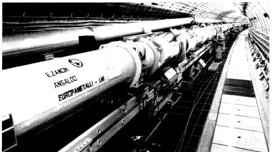
After initial tests with protons in the superconducting ring (above), commissioning of the 6.3-kilometre HERA electron-proton collider ring at the DESY Laboratory in Hamburg switches to electron beams.
